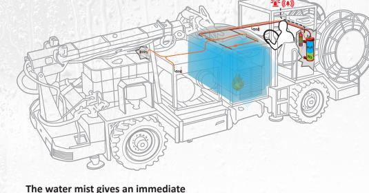
choking and cooling effect. It fills the entire fire-protected compartment and accesses fire beds even outside the direct spread of the nozzles.
