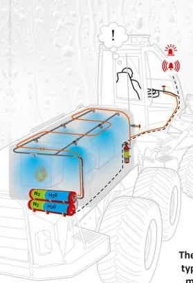
The Fogmaker system is tailored for each type of machine. It is important to us to make a risk analysis together with the customer prior to installation.
