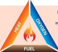
Fogmaker's fire suppression system handles all three sides of the fire triangle: heat, oxygen, and fuel. The system deploys when the protected area becomes too hot, and sprays a water-based mist that expands and chokes the fire. The mist also cools the area for a long time - at least double compared to other certified systems\* - which prevents reignition.
