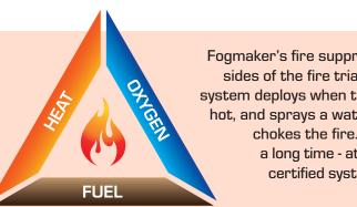
Fogmaker's fire suppression system handles all three sides of the fire triangle: heat, oxygen, and fuel. The system deploys when the protected area becomes too hot, and sprays a water-based mist that expands and chokes the fire. The mist also cools the area for a long time - at least double compared to other certified systems\* - which prevents reignition.
